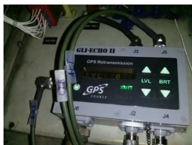
Abb. shows gnss repeater for GPS L1 and L2 in a Lockheed Martin C-130 Hercules
