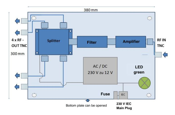
System: Cabinet GPS signal distribution with Filter, Amplifier, Splitter 1 in 4, Housing Protective class I
