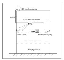
This Repeater GPS System is designated for transmission of GPS signals within buildings like factories, laboratories, testing benches, production halls, EMI chambers and alot more. Please run the system only in closed rooms. Please ask your federal office if you have any questions about retransmission of GNSS
