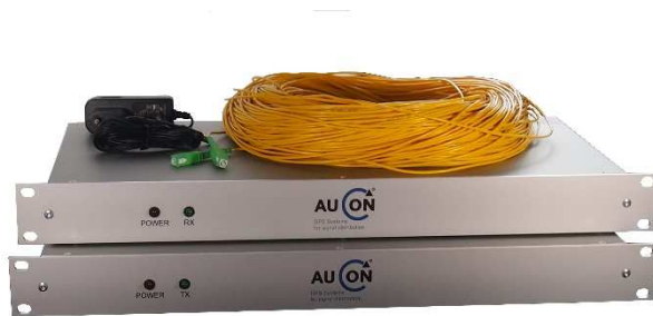
Picture above: conversion of the RF signal into light waves in a wall cabinet housing
