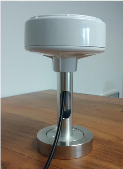
The GNSS outdoor antenna (white) is directly mounted on a flat surface on the roof by means of the provided base and can be encumbered with the weight.
