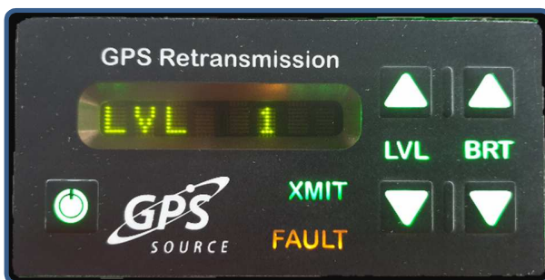
Image 3: LED-display with the system's status information
